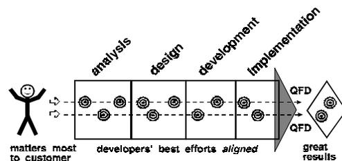
**Figure 4. Coherent Planning and Development.** QFD targets best efforts on value to the customer. For equivalent effort, more value is received.
