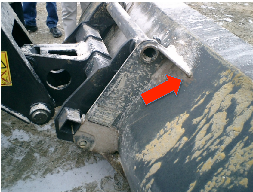
Figure 2 Added welds for extreme applications
